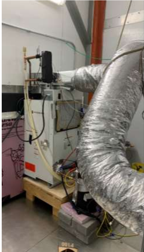
Code tester to measure air flow rate
