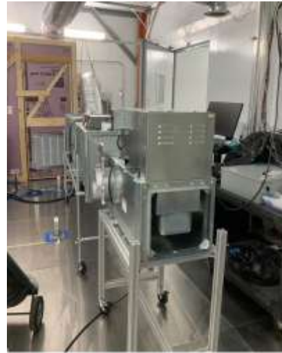
Code tester to measure air flow rate
