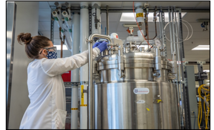
Scale-up to 300L bioreactor for cell-free catalysis
