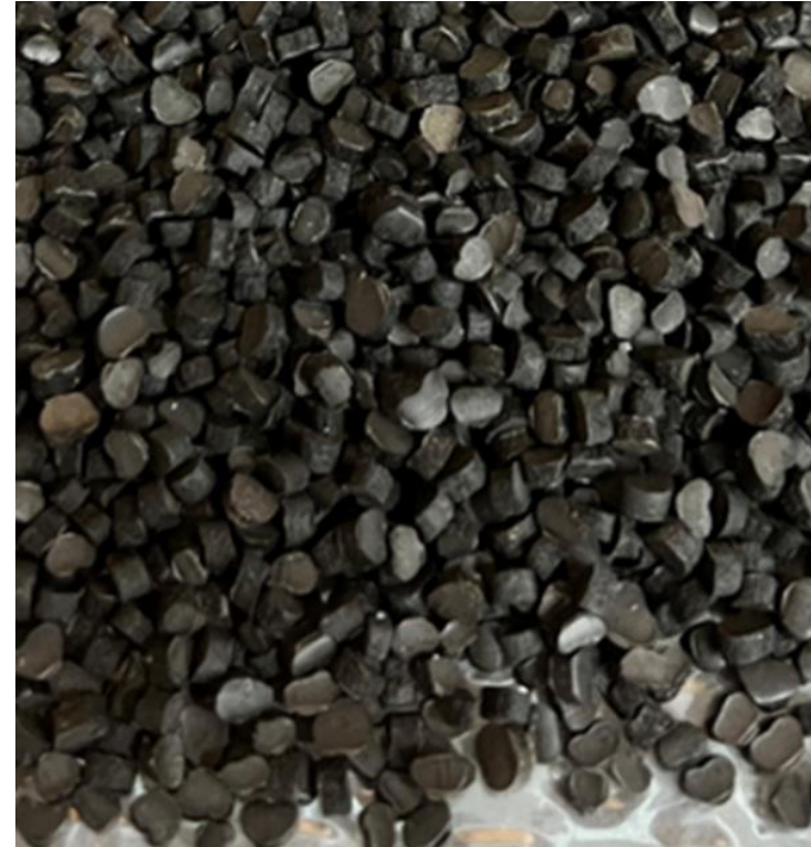
100% Film plastic extruded pellets
