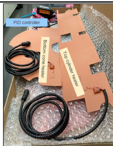
Custom Made Silicone Rubber Heater & PID controller.
