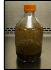
High Solids Hydrolyzed DMR CS
