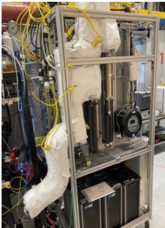
Picture of the condensation system at NREL for collecting vapors from coking pyrolysis oils (cold finger, condenser, electrostatic precipitator, GC analyzer).
