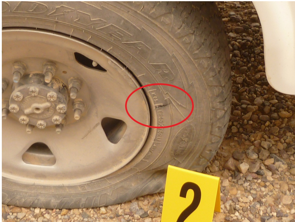
Figure ES-4. Tire Punctured by Shrapnel from Drum Explosion
