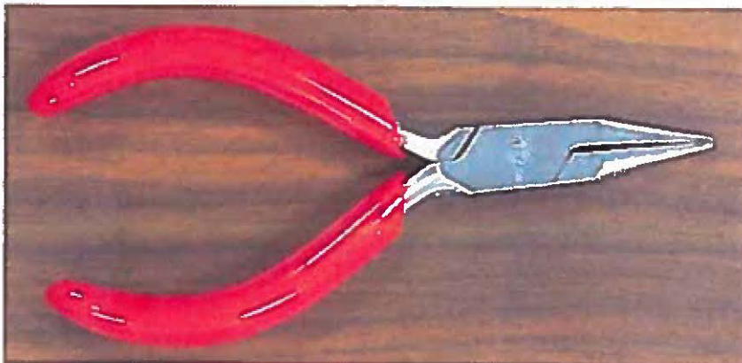
Figure C. A pair of needle-nose pliers such as this is the tool specified for o-ring extraction.
