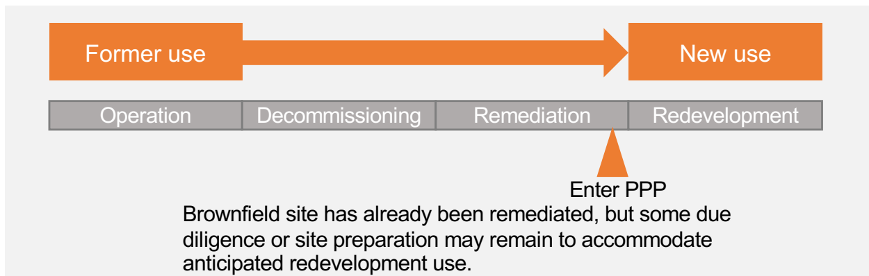
Figure 9: PPP at later stage of redevelopment process.
