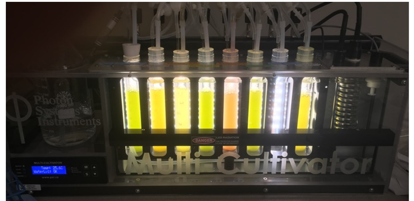
Lab-scale cultivation system of algae identified by the DISCOVR consortium
