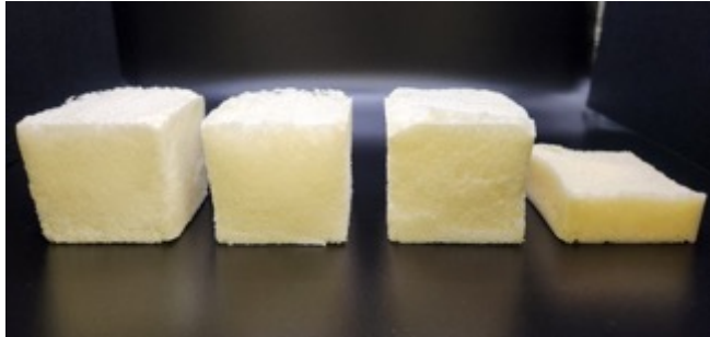
(Left to Right) 0, 10, 30, 50% Polyol Replacement with Pyrolysis Oils
