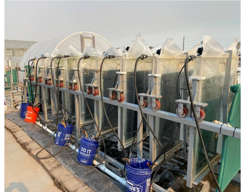
Figure 1 MM FP-PBR setup for the Summer 2021 run. Nine (9) reactors in total were used in groups of three (3) with one of each strain per group.
