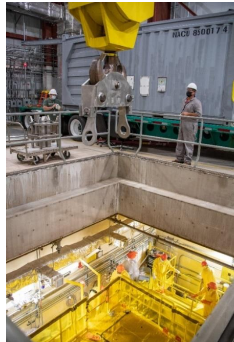
The SRS Tritium Extraction Facility performs a cask receipt, enabling TPBARs to be moved safely from shipping casks to basket.
