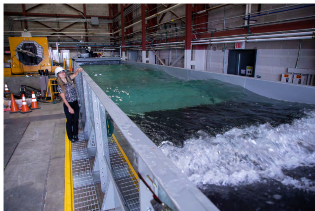
The National Renewable Energy Laboratory's new wave tank will enable early-stage, proof-of-concept testing for wave energy devices. Image from Joe DelNero, National Renewable Energy Laboratory
