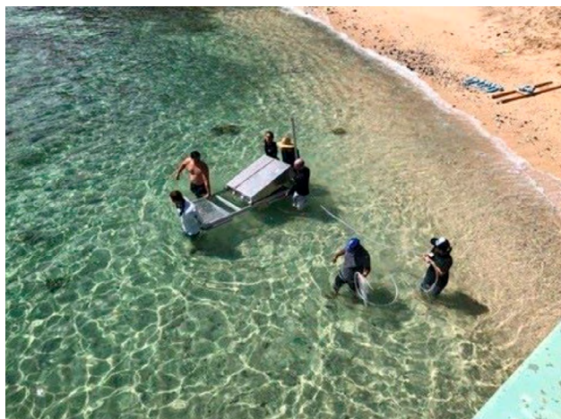
University of Hawaii researchers took their oscillating wave surge energy converter prototype for a trial run in the shallow waters off Hawaii's Makai Pier. Image from Patrick Cross, University of Hawaii
