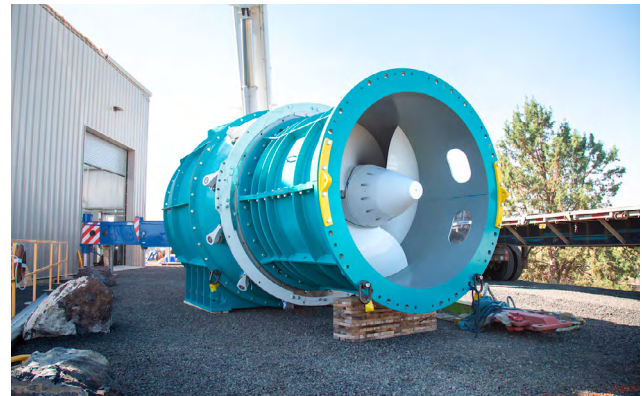
Natel Energy's Restoration Hydro Turbine is designed to make it easier for fish to navigate through hydropower facilities without getting hurt. Image from Natel Energy
