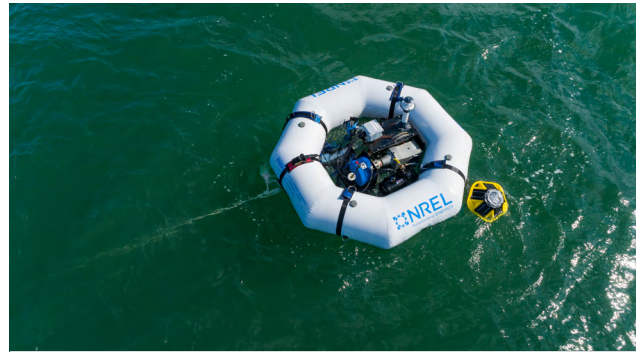
As the National Renewable Energy Laboratory’s first marine-powered desalination device to weather real ocean waters, the Hydraulic and Electric Reverse Osmosis Wave Energy Converter signals significant advancements for marine renewable energy and desalination technologies. Photo from Coastal Studies Institute
