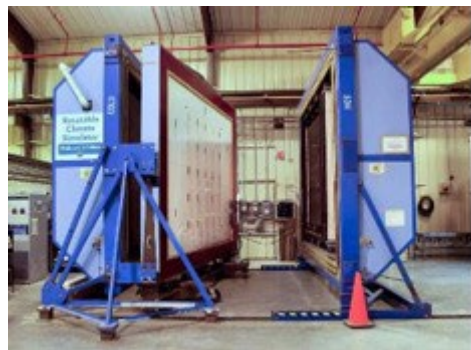
ORNL Guarded Hot Box
