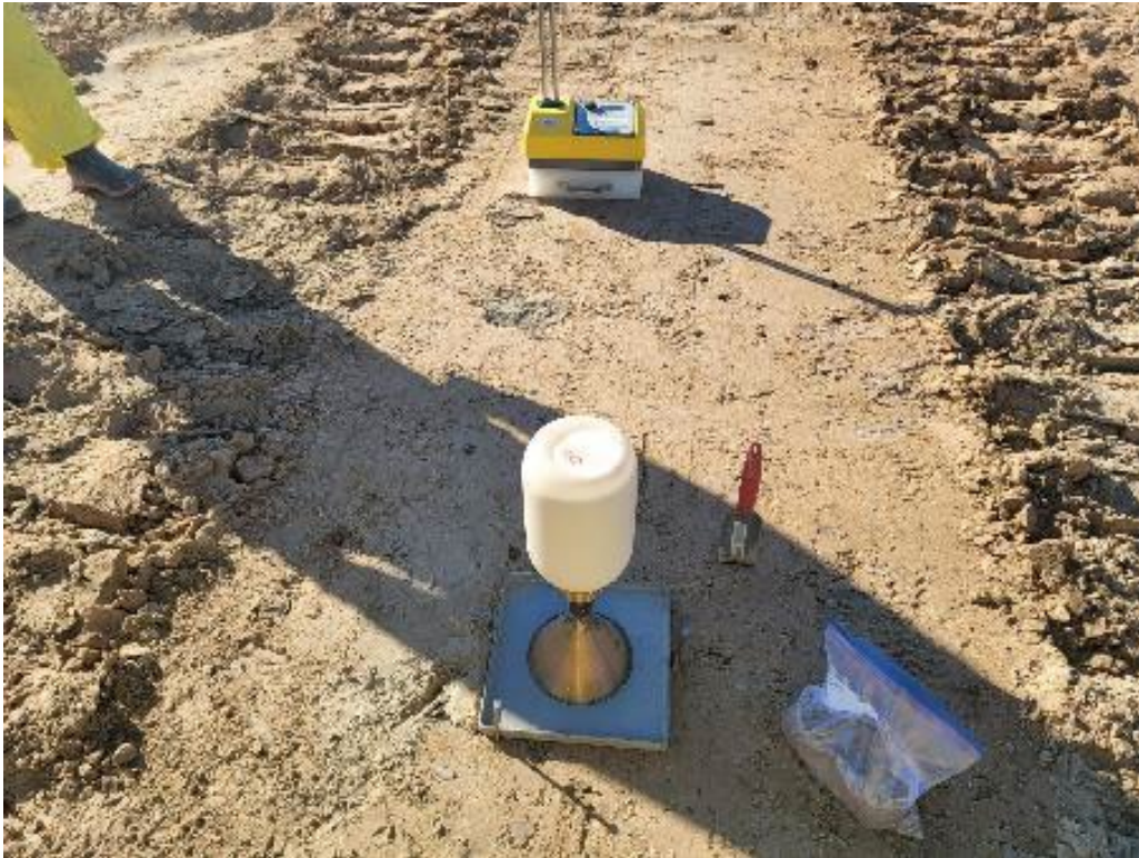
Photo 31. Sand Cone Testing March 2022
