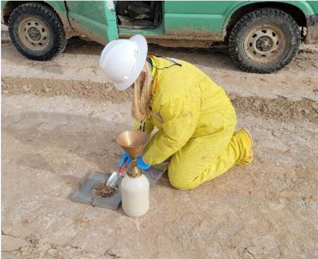
Photo 15. Sand Cone Testing December 2021
