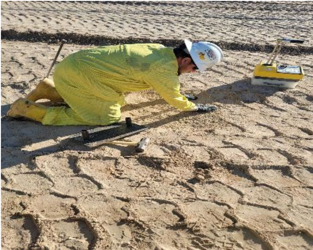
Photo 10. Preparing for Moisture Density Test November 2021
