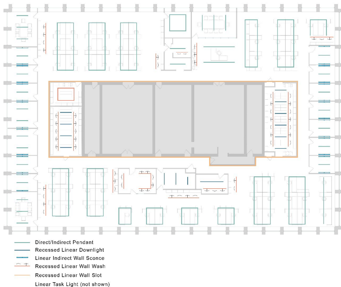
Figure 5. Lighting layout on the 23rd floor. Direct/indirect linear pendant luminaires were arranged in a rectangular pattern over the cubicles in the open office spaces and recessed linear wall wash and slot luminaires were used to increase indirect contributions of light to the eye of occupants. The same pendant luminaires were centered in the private office spaces, with linear indirect wall sconces illuminating two of the office walls. Recessed linear downlights and wall wash luminaires were used in the storage spaces.
