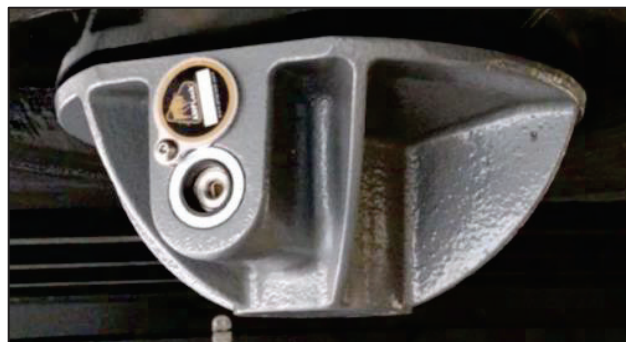
Figure 2. Kingpin Lock Shroud
