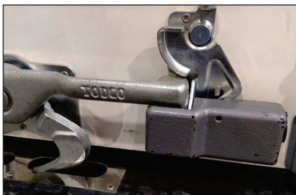
Figure 4. Rear Rollup Door and Lock Shroud
