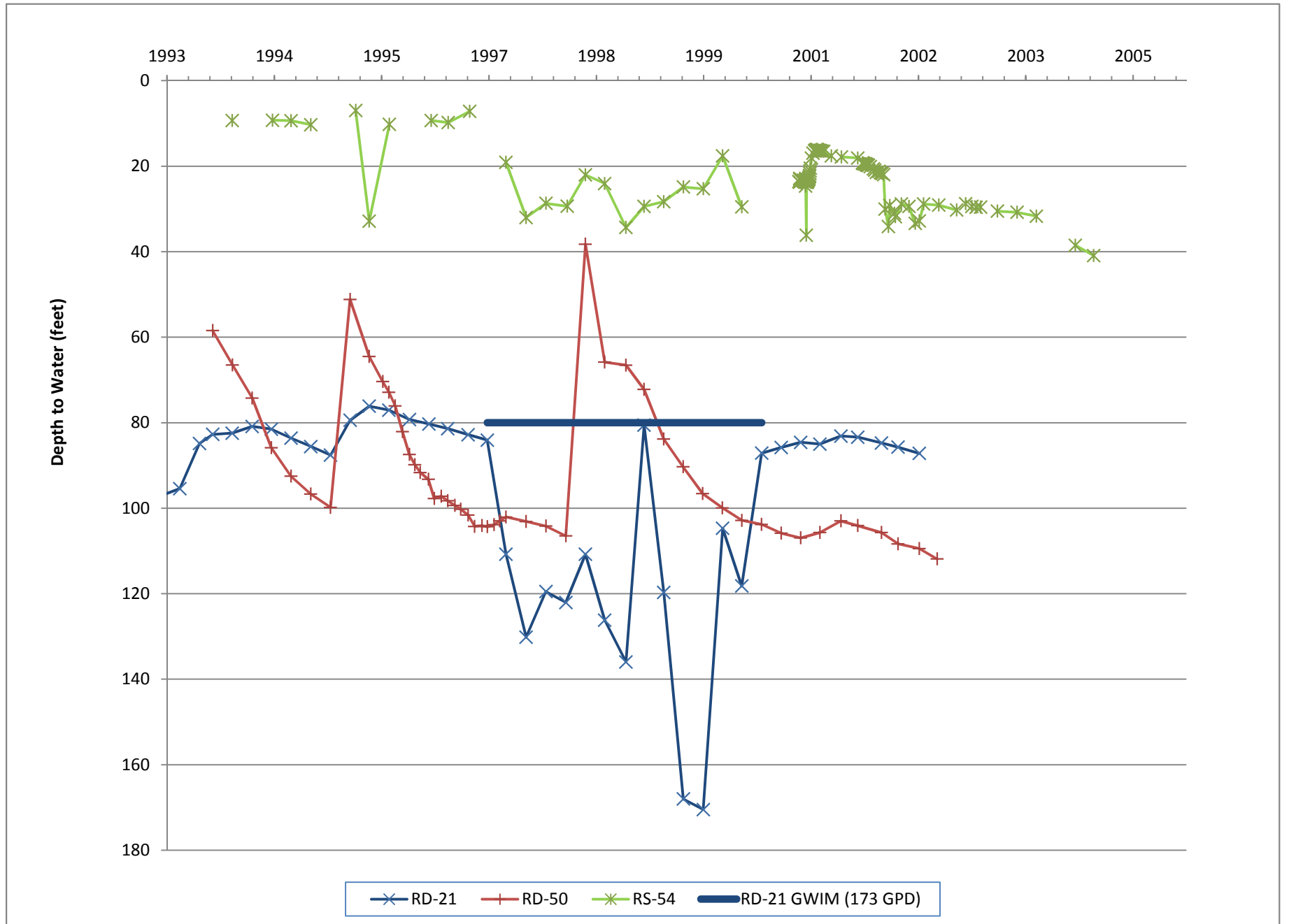
Figure 4-4 RD-21 Pumping - RD-50 and RS-54 Drawdown
