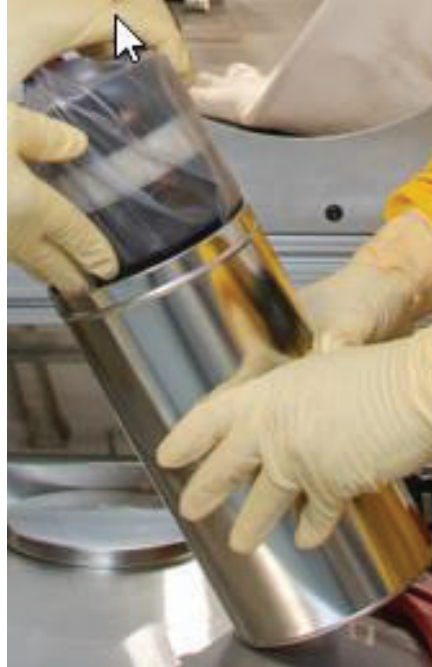
Figure S-12. Diluted Plutonium Oxide CH-TRU Waste Packaged in a Can/Bag/Can
