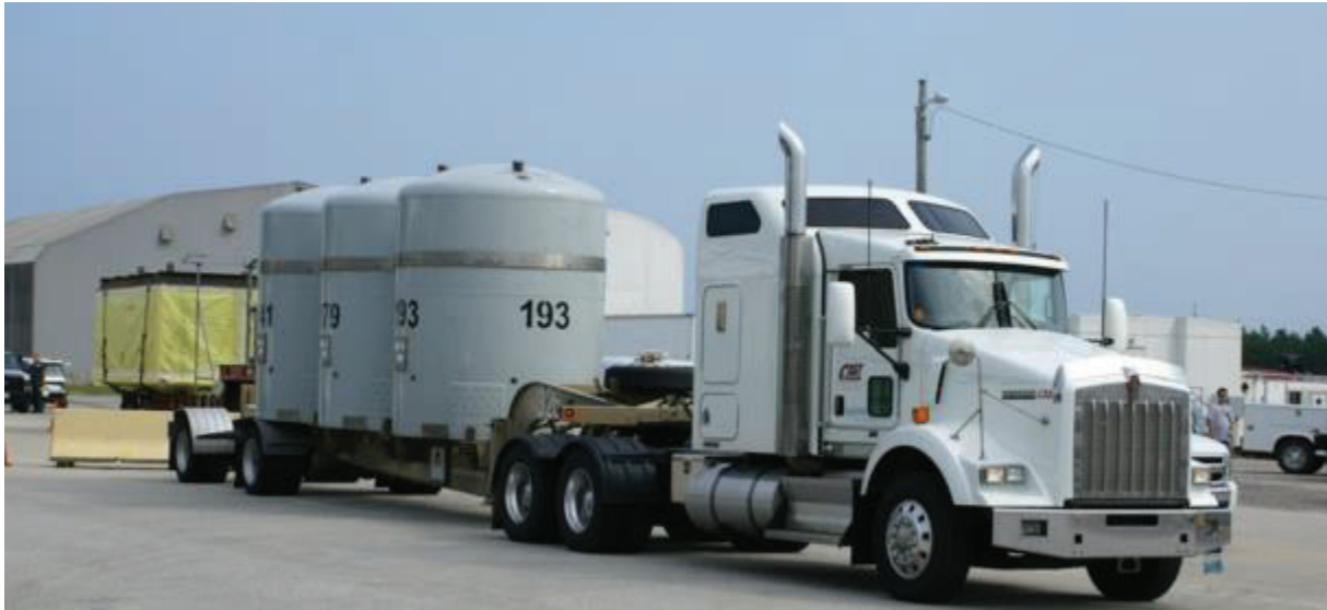
Figure S-15. TRUPACT-II Transporter Used for Shipping CH-TRU Waste to the WIPP Facility
