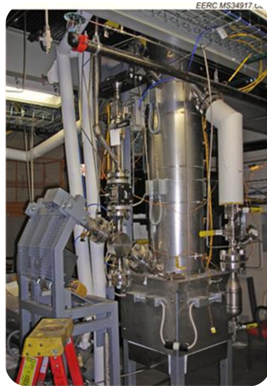
Pressurized Fluidized-Bed Gasification (PFB)
