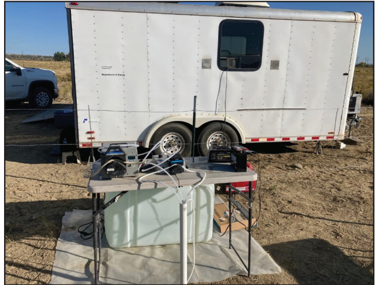
Exterior of the mobile lab during groundwater tracer testing.
