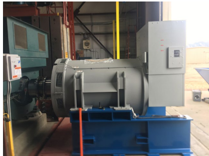
2.2 MVA synchronous machine installed on NREL 2.5 MW dynamometer
