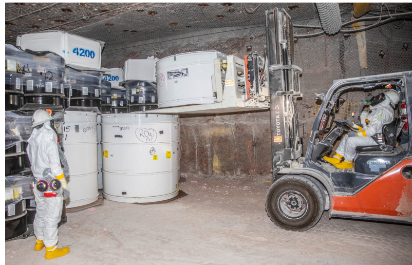
Waste handlers in WIPP's Panel 7 use a push-pull device on a forklift to lift and slide a container into place.
