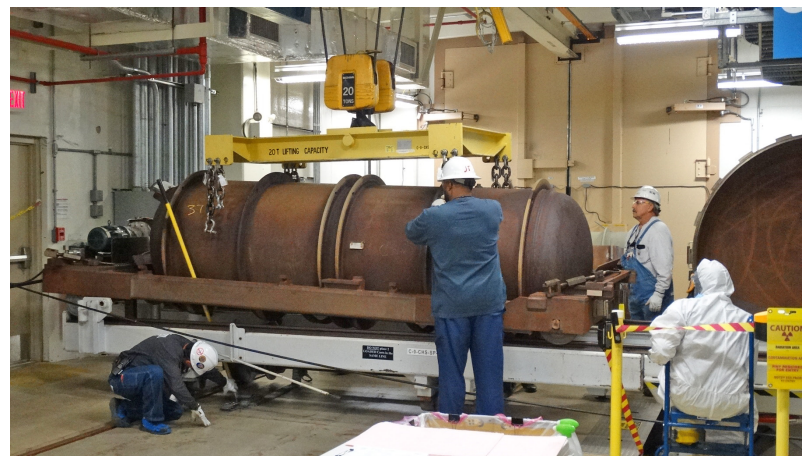
Crews load a non-standard CV-12 cylinder into the Cylinder Transfer System autoclave.
