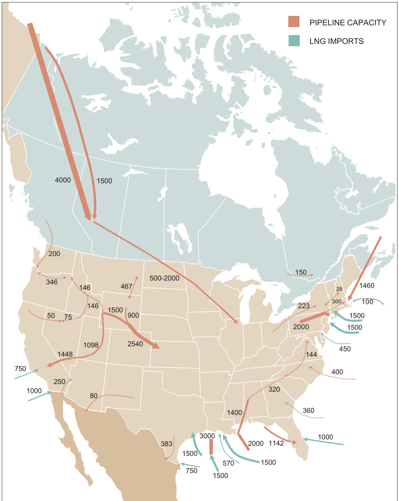
Figure 40. New Pipeline and LNG Capacity (Million Cubic Feet Per Day) Change from 2003 to 2025
