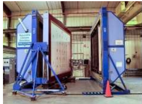
ORNL Guarded Hot Box
