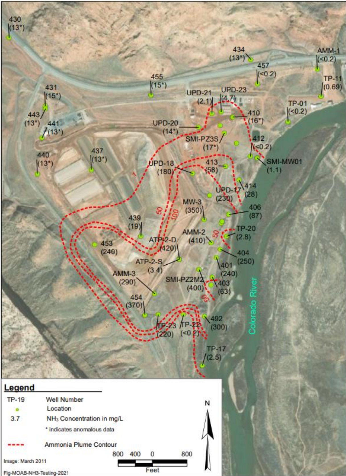
Figure 4. Ammonia Plume in Shallow Groundwater May/June 2021
