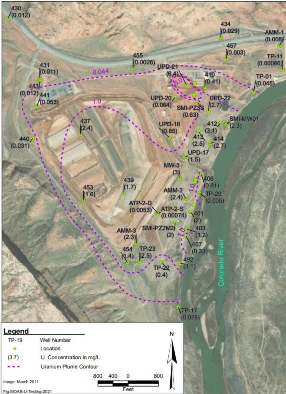
Figure 5. Uranium Plume in Shallow Groundwater May/June 2021
