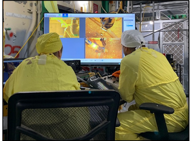
Debris removal inside the General Purpose Cell (GPC) conducted by remote-controlled tools
