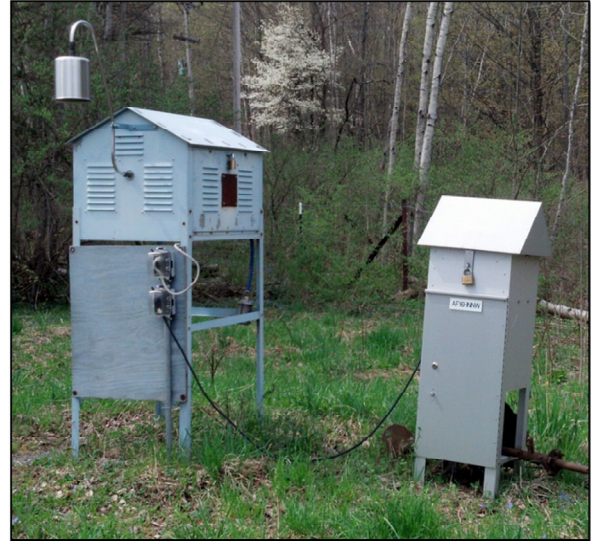
Low-volume (left) and high-volume (right) samplers located in the historical predominant downwind direction from the site
