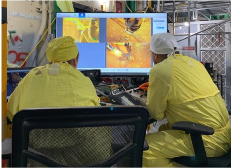
Operators size-reduce debris inside GPC
