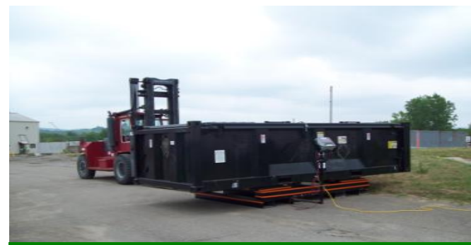
Preparing Intermodals for D&D Activities and Loading of Newly Generated LLW
