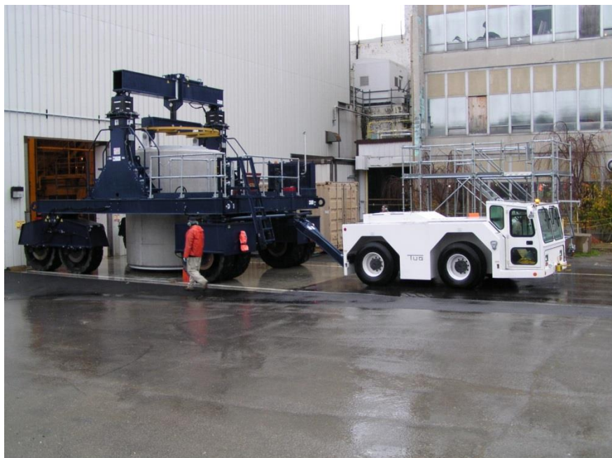
1 st Cask Loaded onto Vertical Cask Transporter
