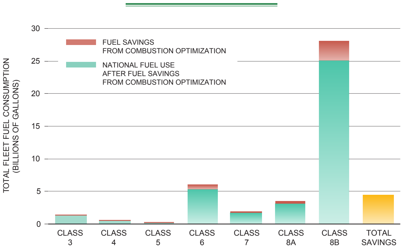
Figure 4-15. Impact of Combustion Optimization on Total Fleet Fuel Consumption (Assuming 12% Fuel Efficiency Improvement)
