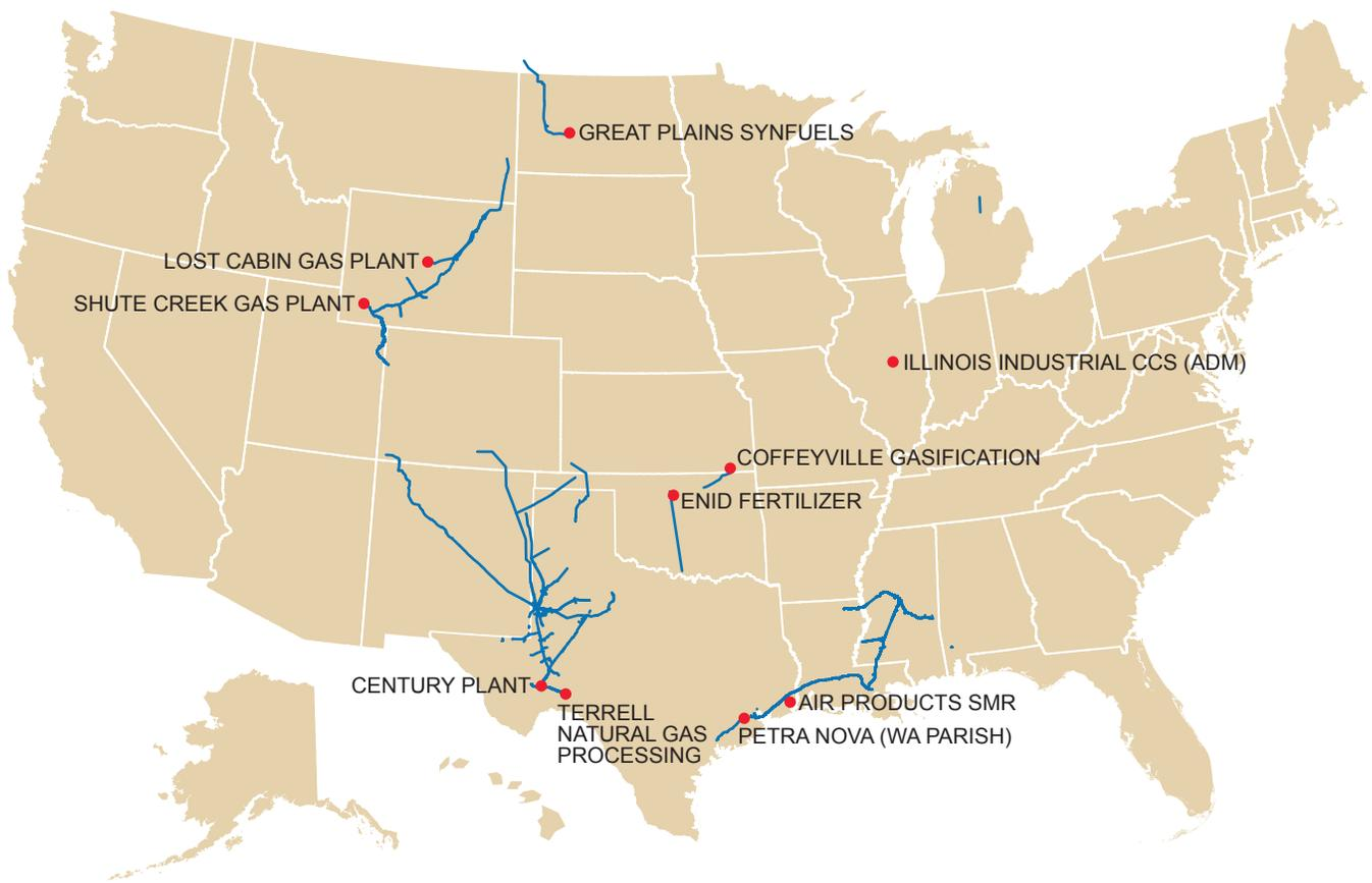
**Figure 6-2.** Schematic Map of CO<sub>2</sub> Pipelines in the United States
