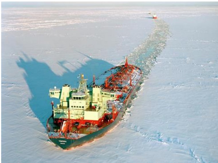
Figure 1. MV Tempera - double acting icebreaking tanker. (Photo: Aker Arctic)
