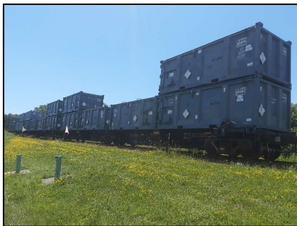
Shipping waste soils off site by rail
