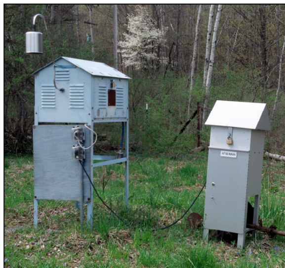
Low-volume (left) and high-volume (right) samplers located in the historical predominant downwind direction from the site
