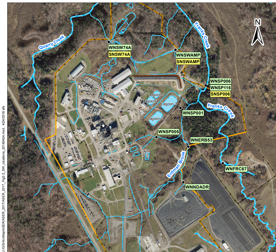
FIGURE 2-2 Surface Water and On-Site Soil Sampling Locations
