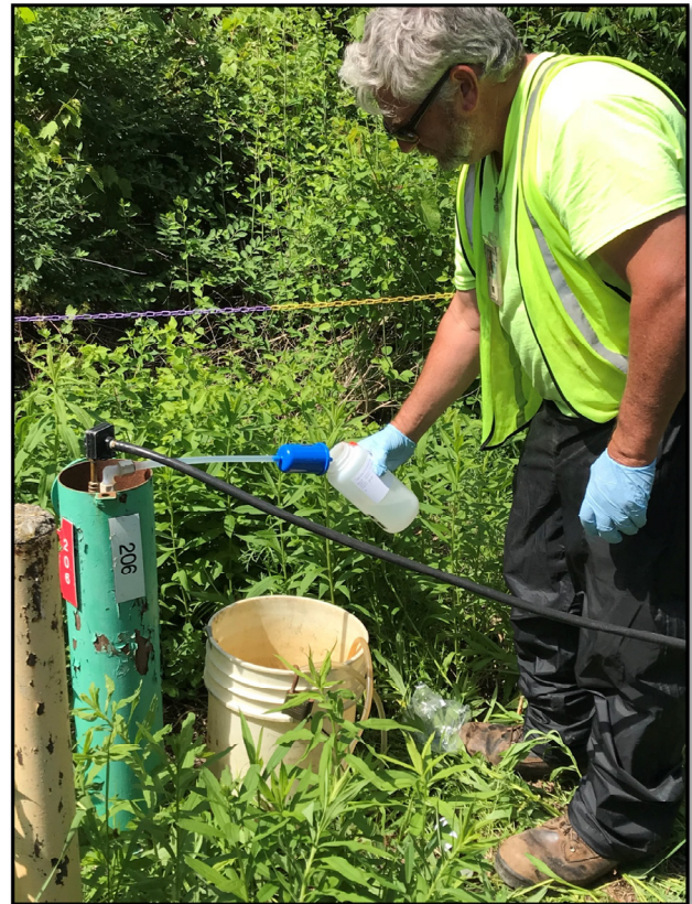
Routine groundwater sampling
