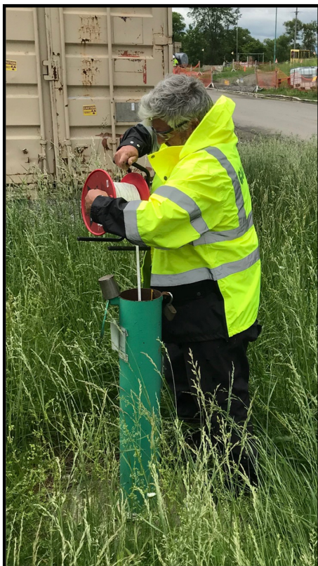
Measuring groundwater elevations
