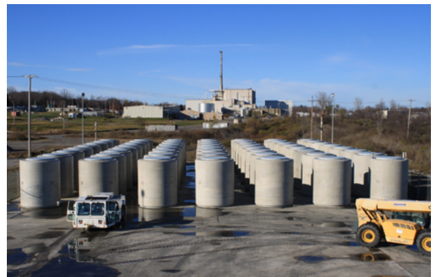
56 Vertical Storage Casks (VSCs) safely stored on site
