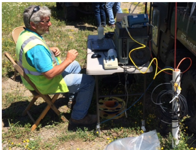
Groundwater bromide tracer test being performed on one of the PTW wells installed in the zeolite
