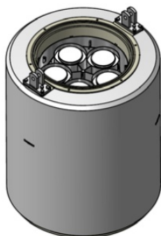
Vertical Storage Cask (VSC) and Overpack
