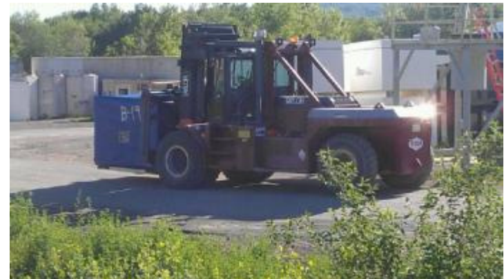
Moving Kistners Containing HEC Drums to Storage
