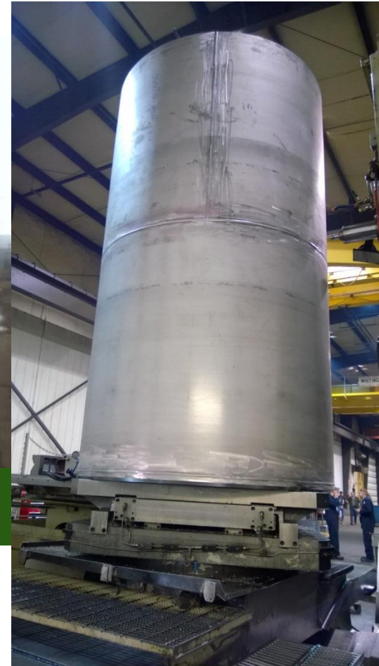
Overpacks Being Fabricated
