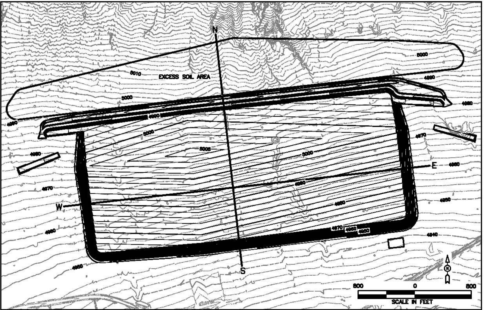
Figure 7-2. Disposal Cell Layout with Typical Cross-Section Locations
