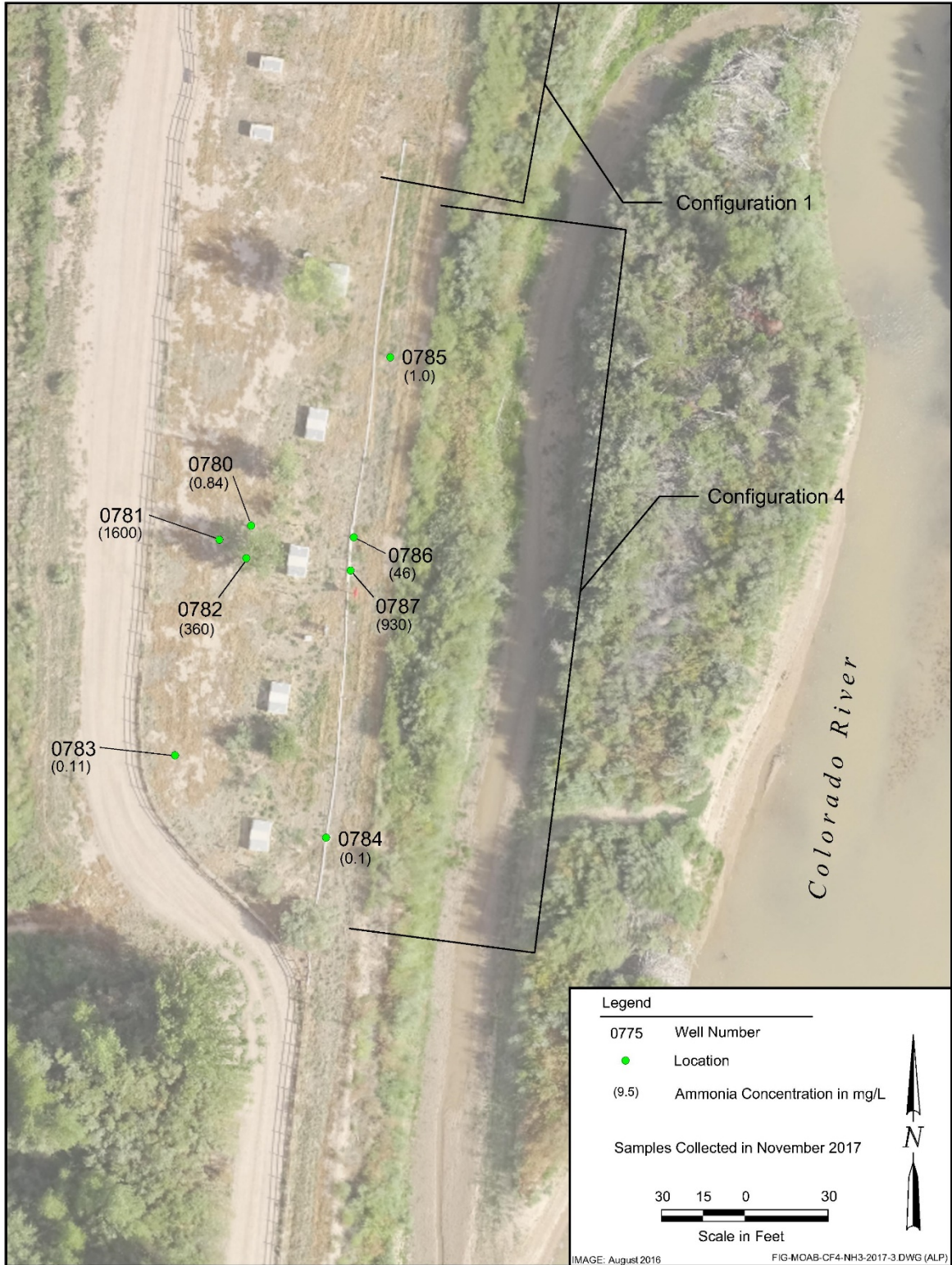
Figure 5. November 2017 CF4 Ground Water Ammonia Concentrations during Injection
