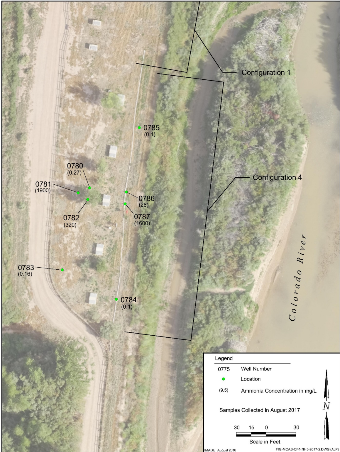
Figure 4. August 2017 CF4 Ground Water Ammonia Concentrations during Injection
