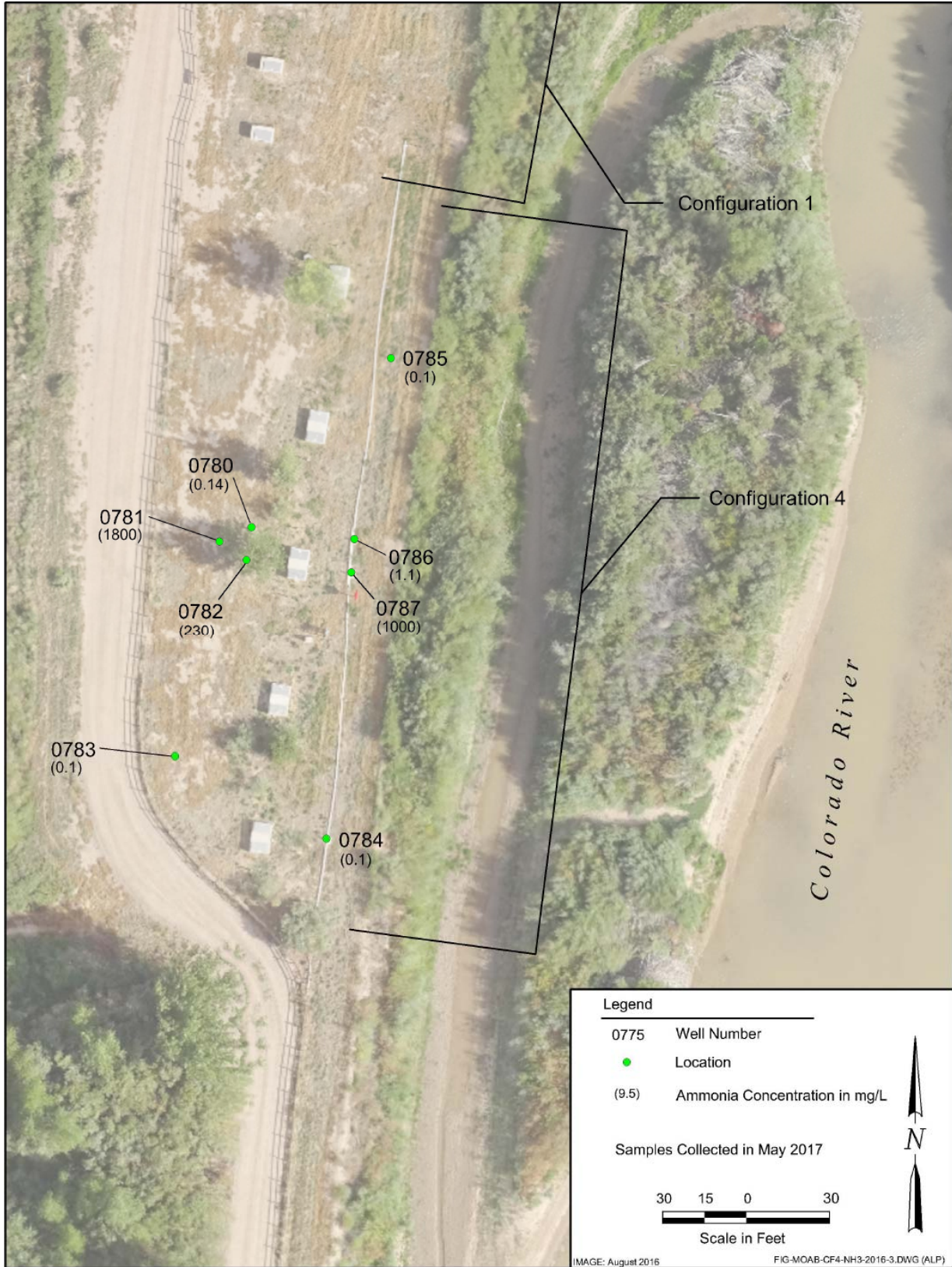
Figure 7. May 2017 CF4 Ground Water Ammonia Concentrations during Injection
