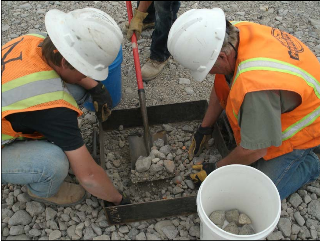
Photo 43. Infiltration and Biointrusion Barrier Gradation Test Sampling June 17, 2011
