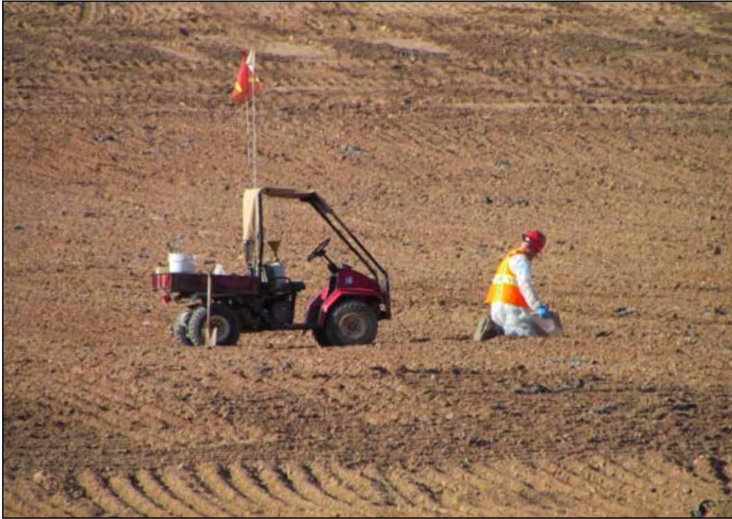
Photo 22. Sandcone Testing August 19, 2011
