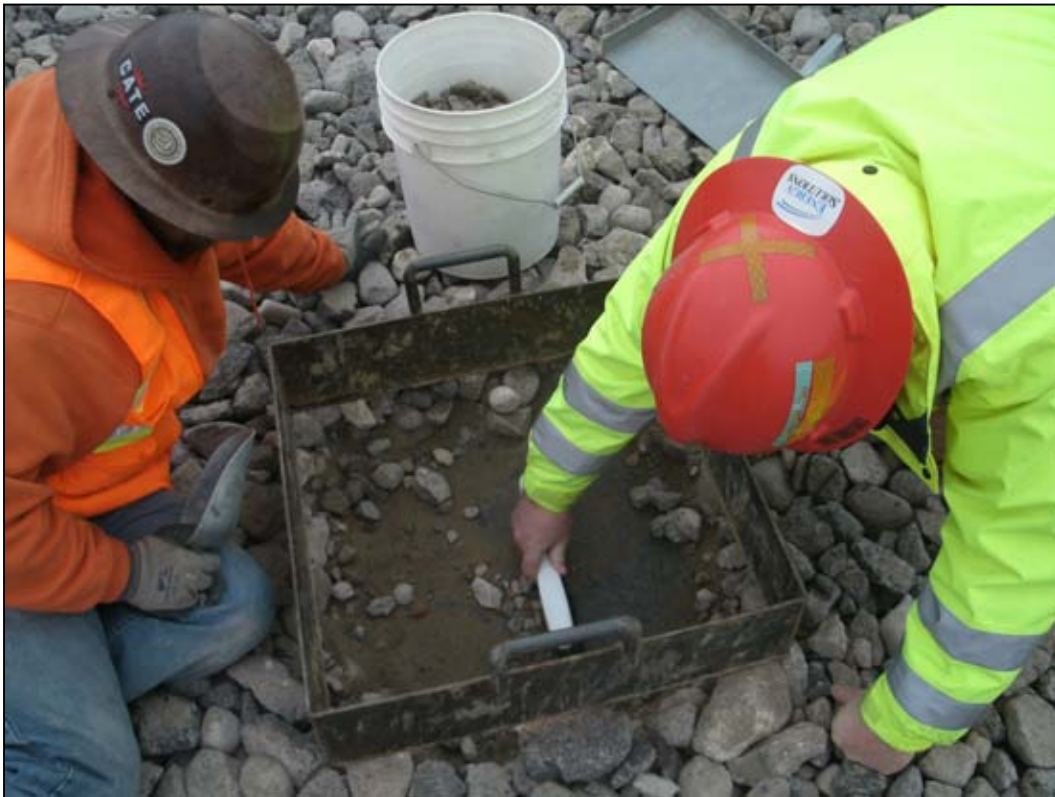
Photo 59. Cap Rock Gradation Sampling December 2, 2011
