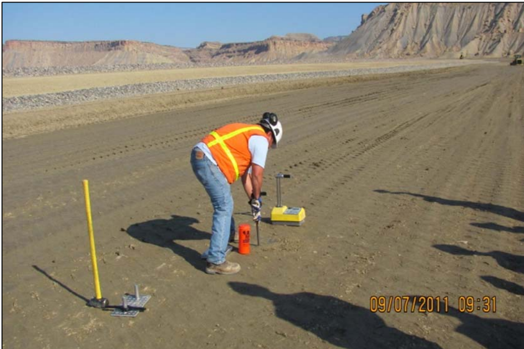
Photo 35. Radon Barrier Independent Testing September 7, 2011
