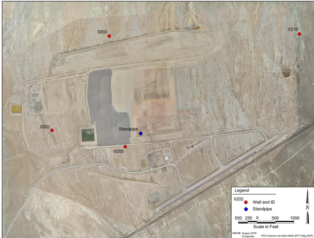
Figure 5. Locations of Monitoring Wells and Standpipe
