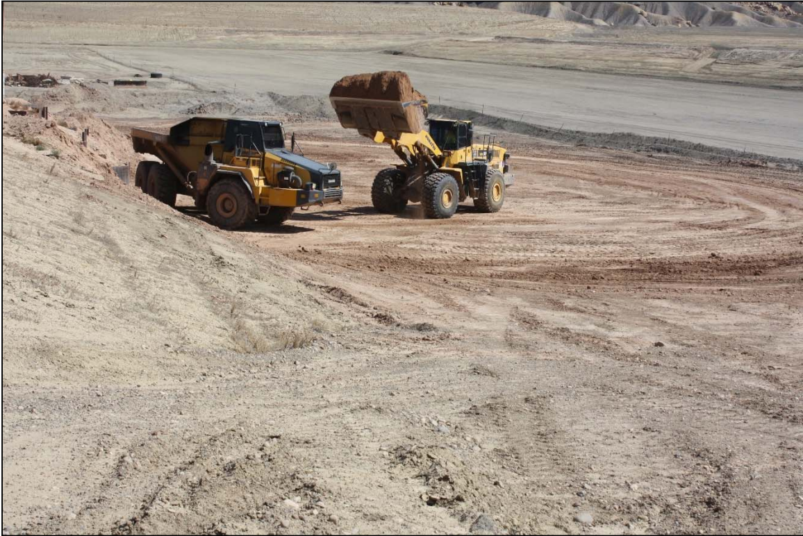
Photo 43. Loader Loading Material in Haul Truck at CA Loadout Area June 2018
