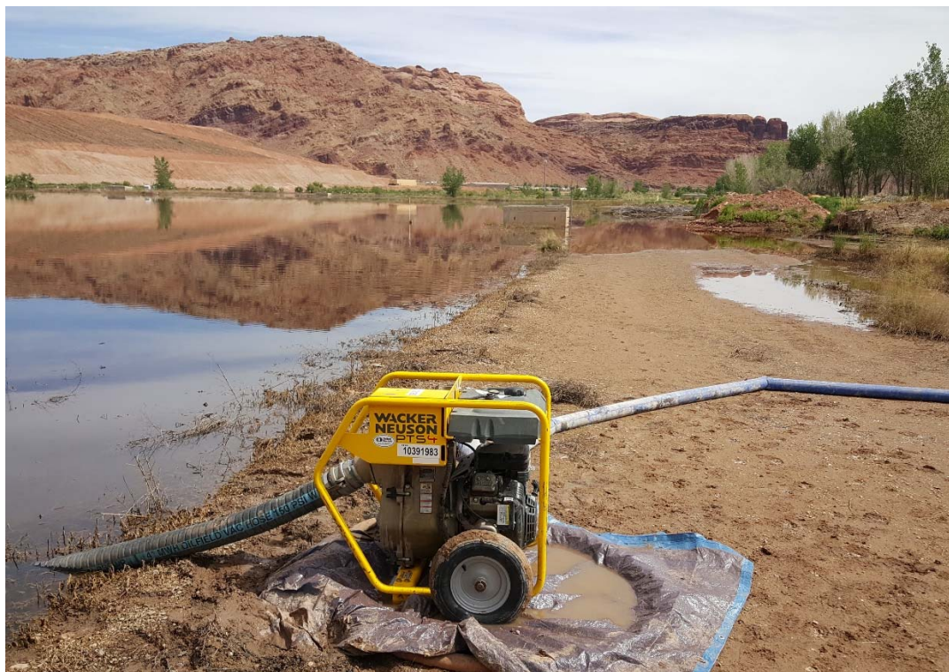
Photo B-25. Trash Pump Transferring Water from Well Field to the Irrigation Plot
