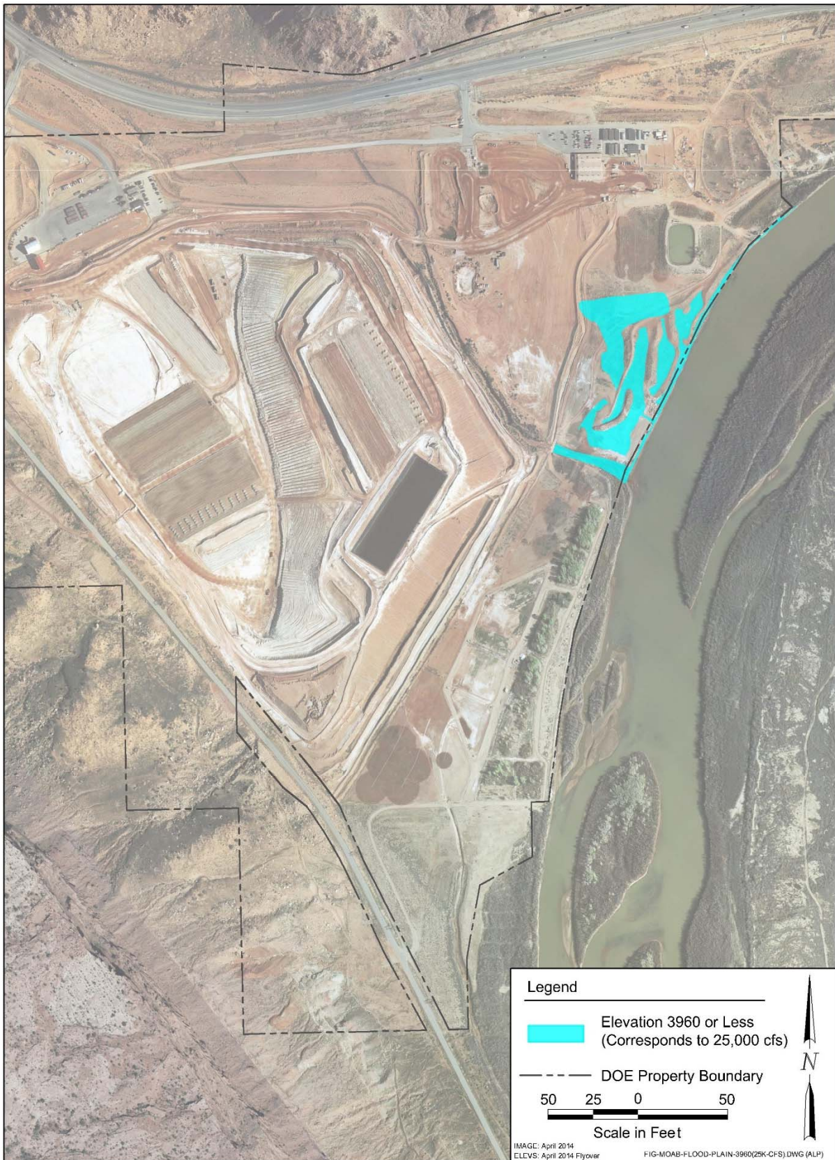
Figure A-2. Floodwater on Site at 25,000 cfs
