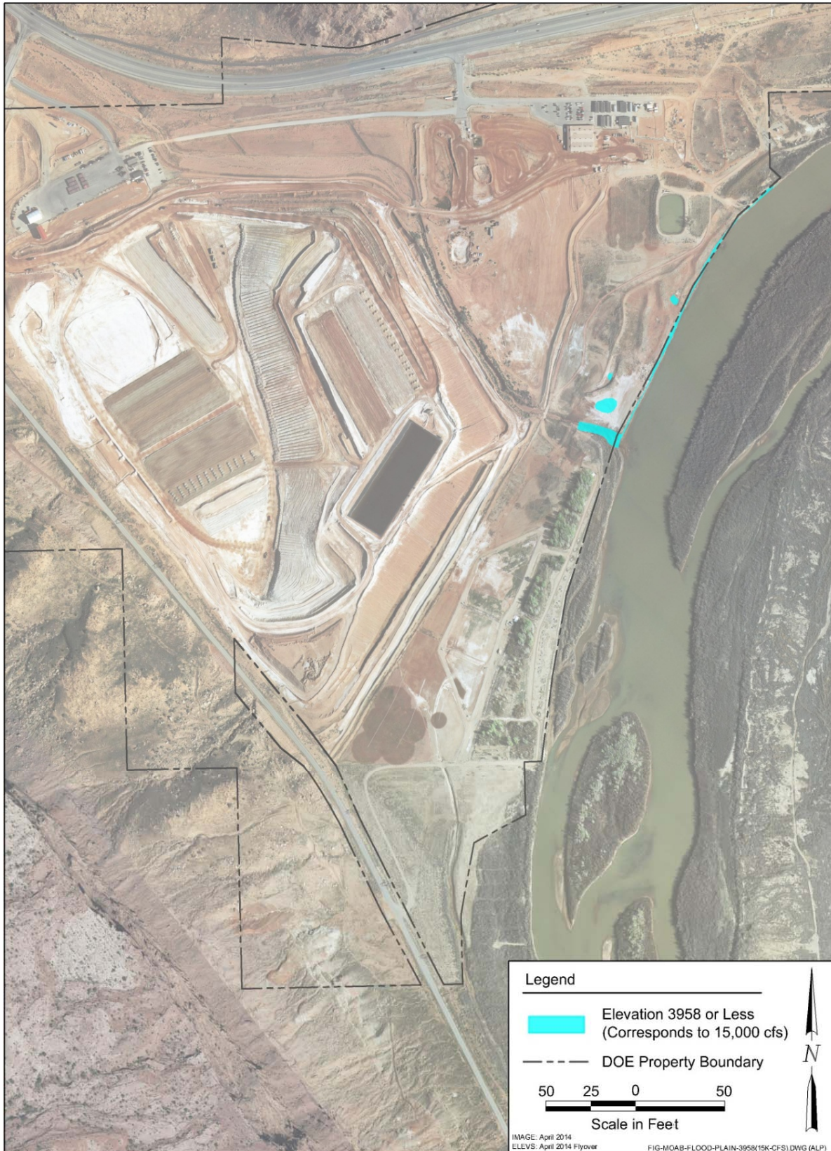
Figure A-1. Floodwater on Site at 15,000 cfs
