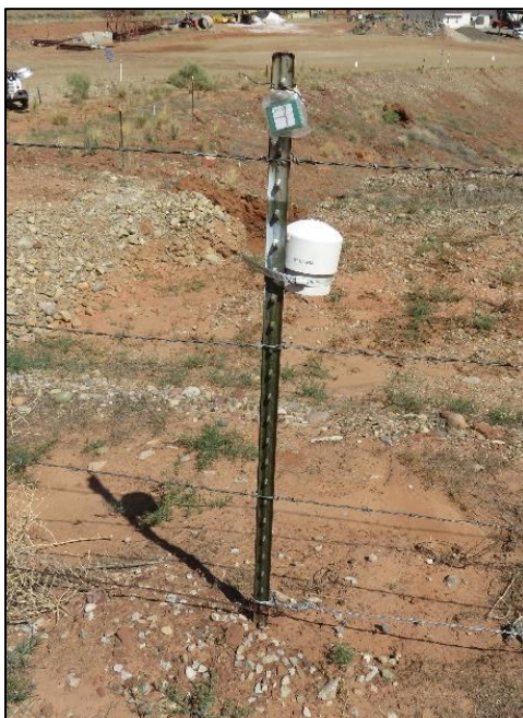
Figure A-1. Example of TLD (top) and Radon Detector Environmental Enclosure
